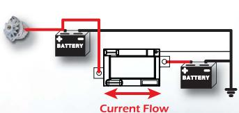
A solid state Bi-Directional Relay can be used to switch power between two batteries. Current can flow in both directions much like a mechanical relay. Reprogrammable logic causes the device to respond to differing voltage and timing cues, safeguarding batteries from deep discharge, or monitoring voltage, current, and termperature for various internal or external battery management applications.
